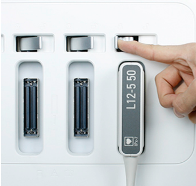
Connecting a Transducer to the System
